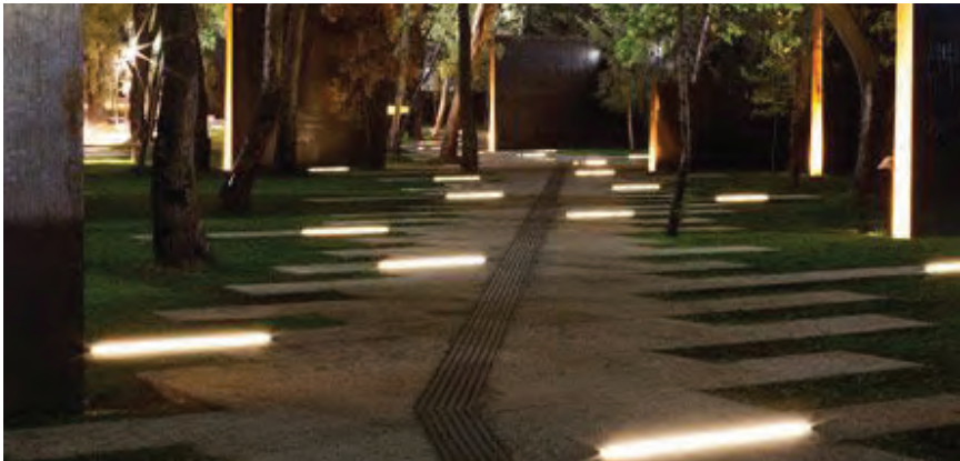
Park Entrances Linear high output LED would be recessed into the paving and vertical surfaces to act as entrance markers. Could also be flexible LED strips taking the shape of indigenous symbols.
